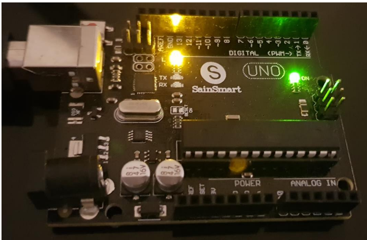
Figure 3-5: Arduino UNO-compatible board with the built-in LED turned on
